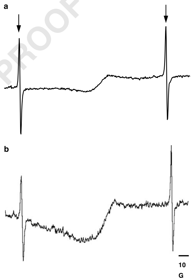
Figure 2 EPR spectra: EPR spectra taken ex vivo at 77 K showing steady-state native free radical concentrations in the cervical spinal cord of (a) exercised and (b) non-exercised rats treated with H 2 O 2 . Spectra containing two Mn/MnO signals as internal standards are indicated by arrows. The area observed between the two signals of standards was double-integrated for evaluation.
